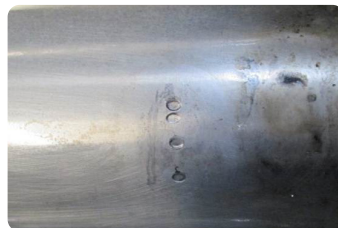
Defect Repair on Blanket Cylinder
